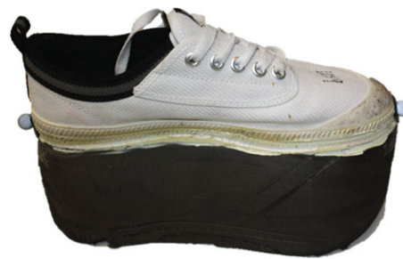
Figure 1. Custom-made platform shoe with an approximately 100 mm additional foam sole. The width of the base was reinforced for safety, providing an additional 20 mm around the middle third of the shoe, with a natural gradient progressing to the most anterior and posterior aspects in a manner such that no additional length was added. (Online version in colour.)
